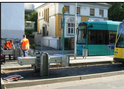
Special design hydraulic buffer stop on an existing rigid buffer stop for city railway cars
