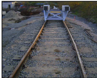
Special design for use in curved tracks.
